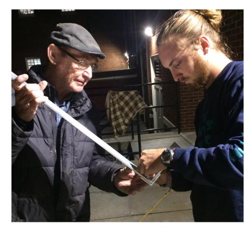
The construction of the frame was simple. We screwed holes in the end of each bar that lined up with the corner brackets in order to bolt the bars together to make a study rectangle. The loops for the pull rope were also bolted directly to the frame. The net is bolted with approximately eight bolts on both the top and bottom.
